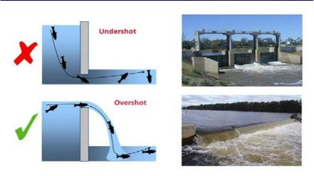
**Figure 14.** More fish survive overshot weirs (lower diagram & photo) compared to undershot weirs (upper diagram & photo).
