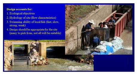
**Figure 8.** The solution: engineered structures that enable fish to overcome the various physical and flow barriers challenging fish passage.
